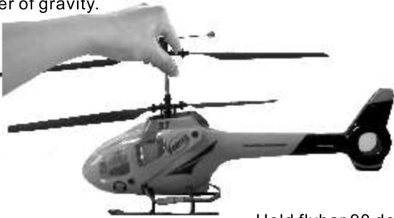
Hold flybar 90 degrees to the tail to test center of gravity.
