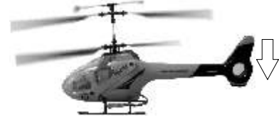
Reducing throttle moves the helicopter lower in the air by decreasing speed to the motors.
